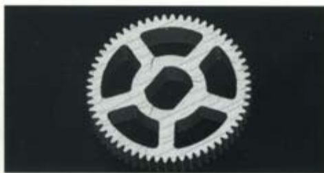
Fig. 1. MEMS LIGA part imaged by DVI technology. Image is an accurate digital replica of all internal and external structures and can be subjected to a variety of visualization and quantitative analysis methods. Source: Dr. Douglas Chinn, Sandia National Laboratories, Livermore, CA.
